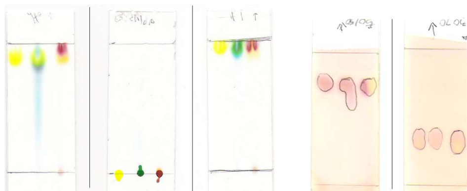
Figure 3. From left to right: Ethanol ink TLC plate, dichloromethane ink TLC plate, 50/50 ethanol/dichloromethane ink TLC plate, 30/70 ammonia/n-propanol TLC plate with amino acid, 50/50 water/n-propanol TLC plate with amino acid. On the amino acid TLC plates, from left to right: Unknown, serine, 50/50 unknown/serine.
